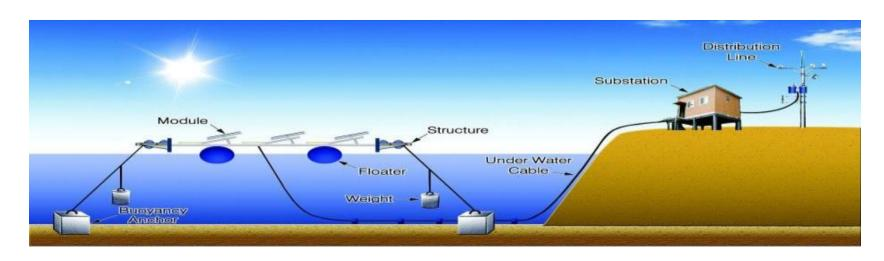
Basically, a floating photovoltaic plant consists of:
